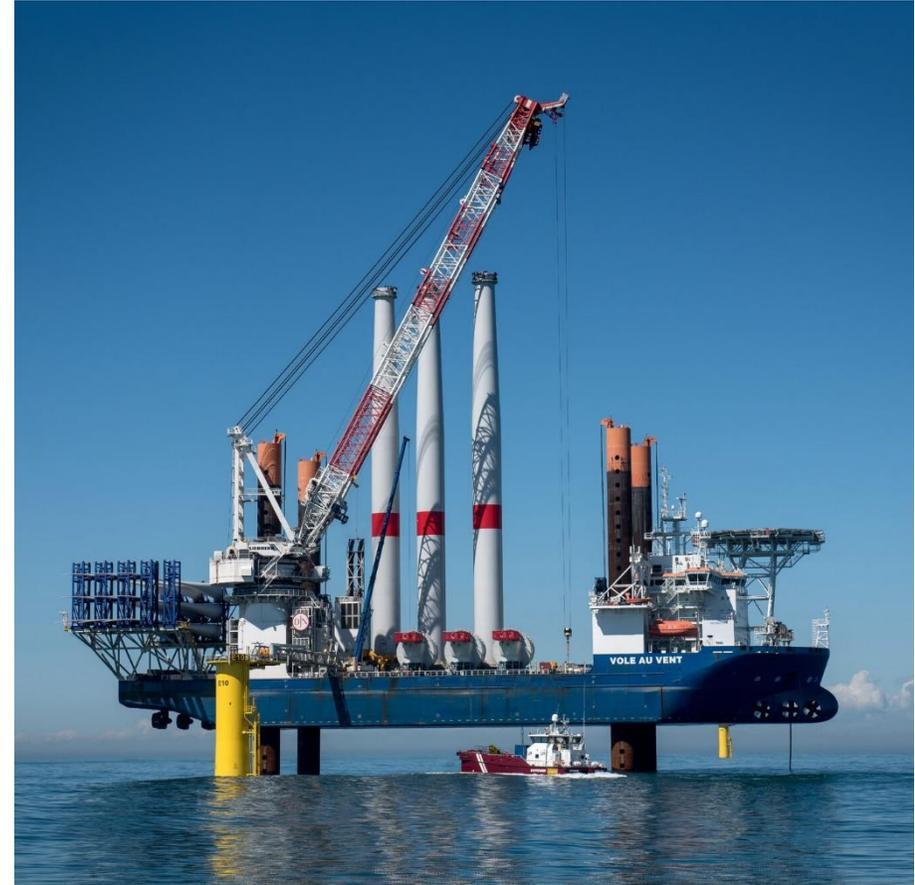
Vole au Vent installing Haliade 6M at EDF Banc de Guerande – St Nazaire
