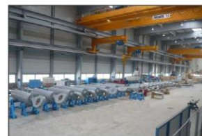
Offshore windmill installation jackup system(2011) 100 DA hydraulic cylinders 650 bore x 320 rod x 2300 mm stroke
